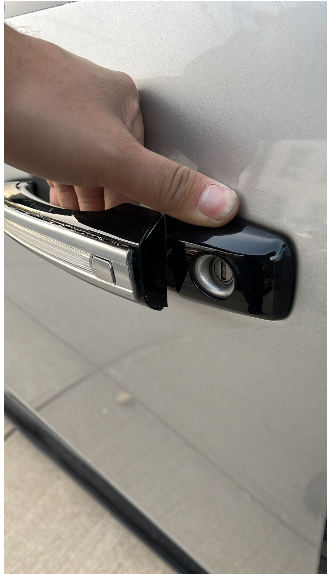
Vinyl overlay placed to cover groove and wire.
